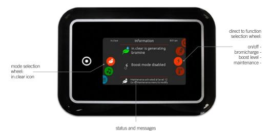
To select the sanitization mode, slide the left wheel up or down until the in.clear icon menu is highlighted in the middle.
